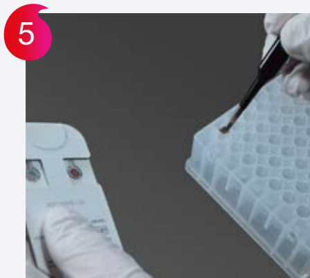
5 Put the disc in a preferred vial, e.g. microtiter plate for subsequent elution.
